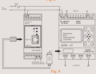
Connection Between Base Module & Communication Module
