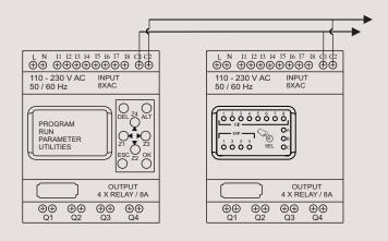
Fig. 3 Connection Between Base Module & Extension Module Same for both AC & DC
